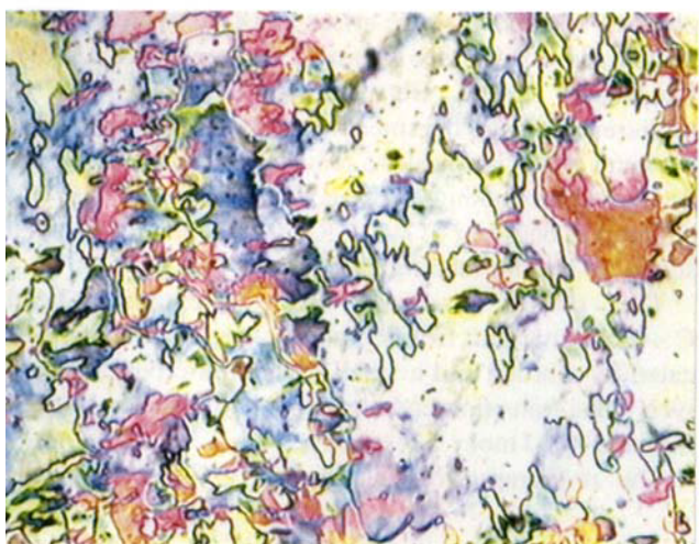
Figure 3. Schlieren texture of the re-entrant smectic C phase of compound DS12 (113°C, magnification: 100 ×).
